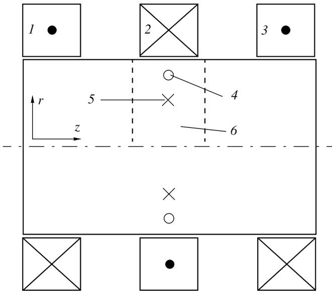
**Fig. 1.** Diagram of the plasma source: (1–3) magnetic coils; (4) an HF antenna; (5) the position of a neutral loop; and (6) the calculation region, bounded by the dashed line.
