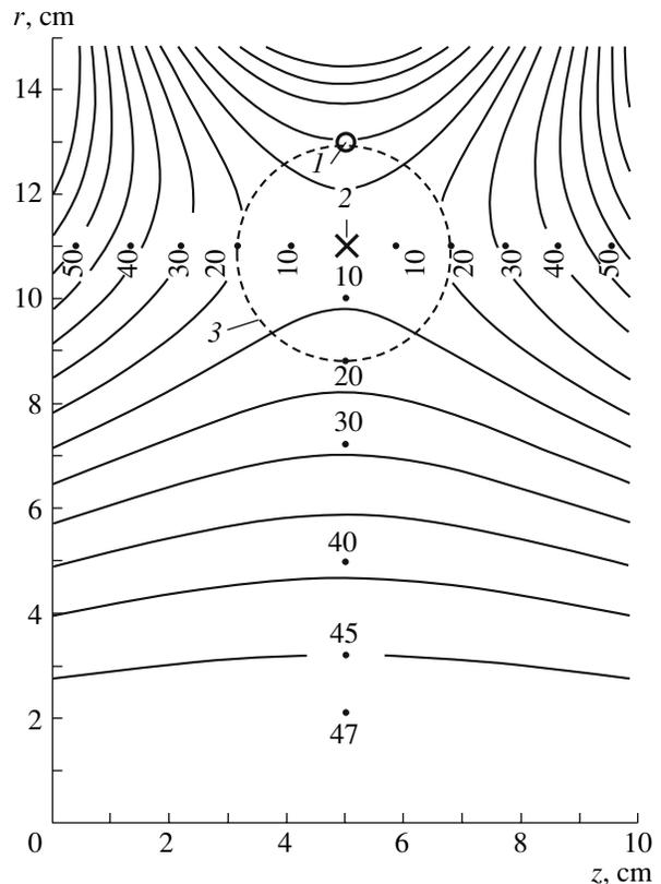
**Fig. 2.** Magnetic-field configuration in the  $(r, z)$  plane: (1) the HF antenna, (2) the position of the neutral loop, and (3) the loop of the magnetostatic field ( $B = 20$  G). The figures on the curves indicate the magnitude of the magnetic induction (in G) at the corresponding points.
