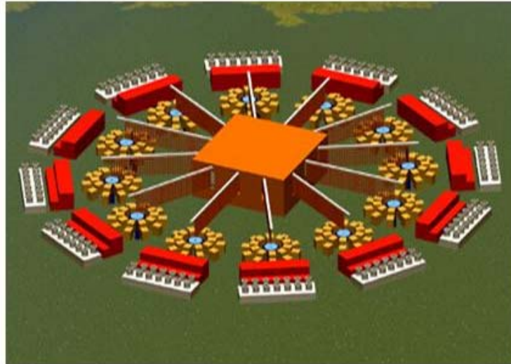
Z-Pinch IFE DEMO (ZP-3, the first study) used 12 chambers, each with 3 GJ at 0.1 Hz, to produce 1000 MWe
